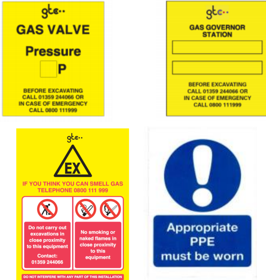
Figure 41 – Examples of the signage required
