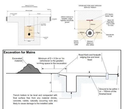
**Backfilling the trench** – this is the responsibility of the Developer unless stated otherwise in the original contract or agreed as a variation during the contract. All cables should be surrounded with cable sand to BS EN 13139.
